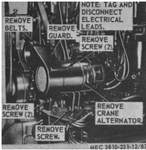
Figure 87. Crane alternator, removal and installation.
