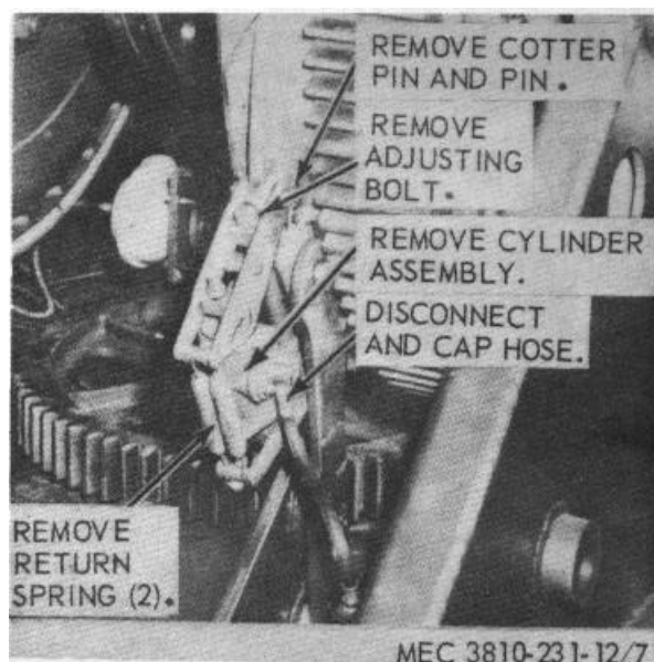
Figure 71. Hydraulic cylinder, removal and installation
