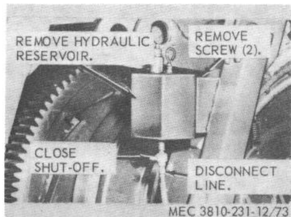
Figure 73. Hydraulic fluid reservoir, removal and installation.
